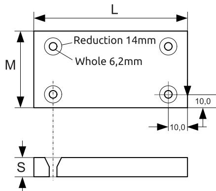
Dimensions head FIBERTEMP FTOSH for Optical Fiber in mm (in)
