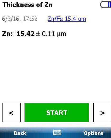
Figure 1. Measurement screen in Coating thickness testing mode.
