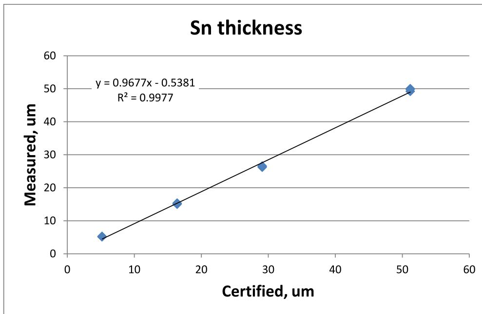
Figure 5. Correlation curve for tin over copper.
