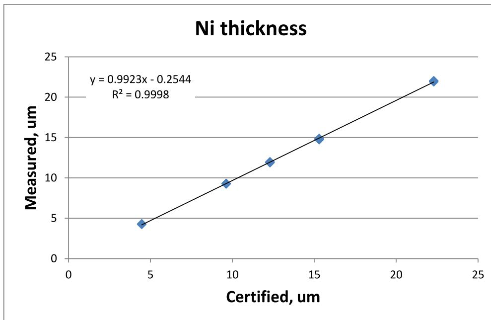
Figure 3. Correlation curve for nickel over iron.
