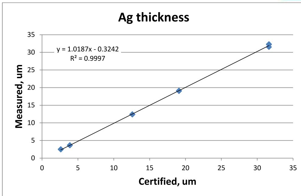
Figure 4. Correlation curve for silver over copper.
