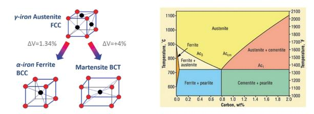
Austenite is a face centered cubic (FCC) phase present in steel at high temperature. Upon cooling, most of the steel is transformed into ferrite - a body centered cubic (BCC) phase – or into martensite – a body central tetragonal (BCT) phase. Depending on the rate of the cooling, some percentage of the steel (typically 0-40%) remains as Austenite. Hence the term "Retained Austenite".
