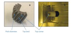
Powertrain samples and measured points (a) and pinion sample mounted on teflon support to measure top corner region (b) taken by inner USB camera.
