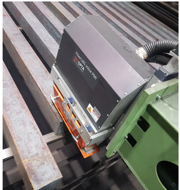
Mix-up control of billets with SECOPTA-sensor
