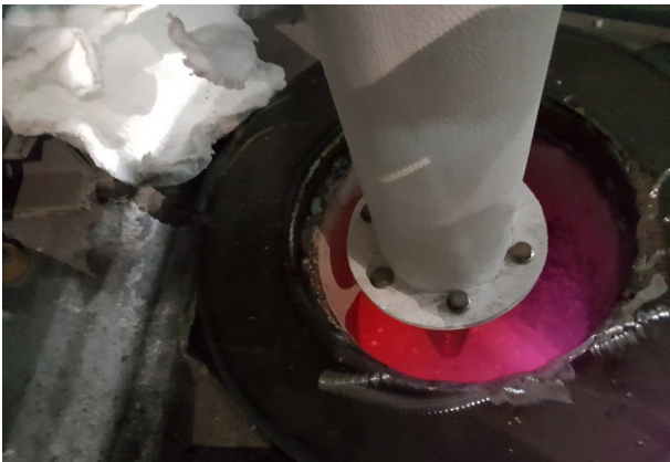
In-situ measurement of aluminum melts
